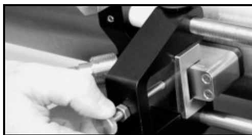
Figure 20: Installing the First Transducer
