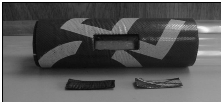
Figure 34: DMP-1 Material with Transducer Footprint Cut Out
