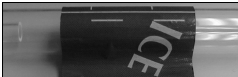
Figure 32: DMP-1 Dampening Material Wrapped Around Pipe
